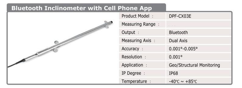
Inclinometers are widely used around the world to monitor the deformation of slopes, embankments, dams, foundation pits and tunnels. By measuring the inclination angle of a sensor probe at different locations inside a casing, we're able to obtain data of soil displacement in vertical or horizontal direction. An inclinometer kit consists of a sensor probe, a mark cable and a datalogger.
