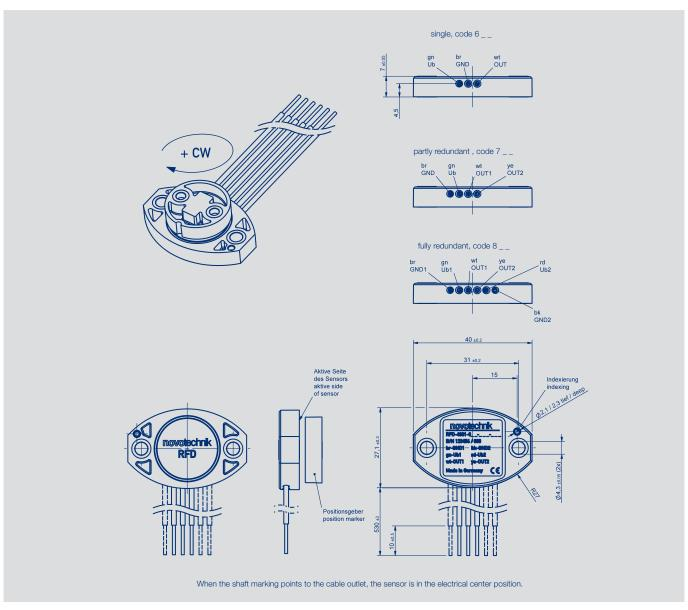
Pin assignment Colour single code 6 \_ \_ partly redundant code 7 \_ fully redundant code 8 \_ Supply voltage +Ub 1 Green Supply voltage + Ub Supply voltage +Ub Brown GND GND GND 1 White Output Output 1 Output 1 Red Supply voltage +Ub 2 Black GND 2 Yellow Output 2 Output 2
