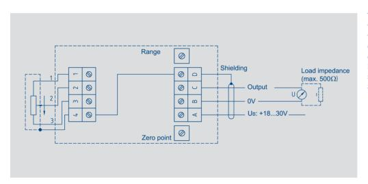
The output signal rises when the wiper is moved from position 1 to 3 (see connection diagram in the corresponding data sheet).
