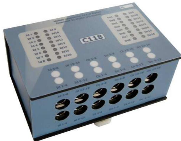
*The C118 is a digital channel expansion unit for datalogger TMF500; it has **16 opto-isolated digital inputs (up to 1000 Vdc)** for ON/OFF states and **16 open collector outputs (max 50Vdc, 200mA)**. Easily connectable to*
