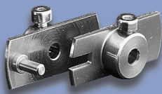
Z 103 G 2.5 Z 103 G 3 Fork coupling with low backlash for shaft diameters 2.5 mm or 3 mm. Stainless steel, ground driving pin. Mounting with 1 fillister head screw M 2 each with hexagon socket. Allen key size 1.5 is supplied.
