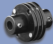
Z 110 G 10 Backlash-free coupling for shaft diameter 10 mm. Black anodized aluminium, driving pin and spring in phosphor bronze. Mounting with 2 threaded pins m 4 each with hexagon socket. Maximum torque 25 Ncm.
