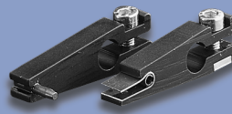
Z 105 G 6 Backlash-free fork coupling for shaft diameter 6 mm. Black anodized aluminium, driving pin and spring hardened. Clamp mounting with 1 fillister head screw M 3 each with hexagon socket. Maximum torque 5 Ncm. Allen key size 2.5 is supplied.
