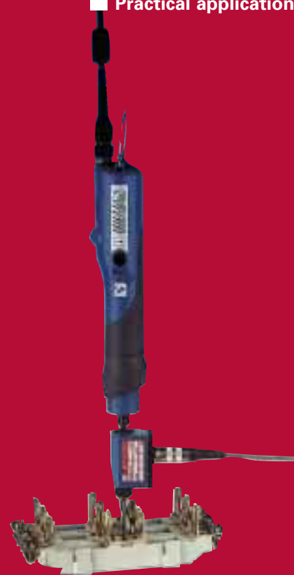
Online torque measurement with screwdriver
