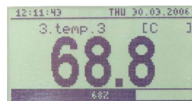
the current value of the measurement signal The height of the digits: 18 mm
